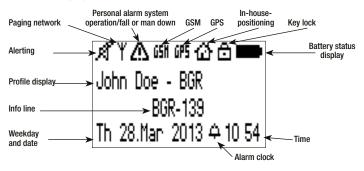
1st line: Status line 2nd line: Profile display 3rd line: Info line 4th line: Date, alarm clock, time
