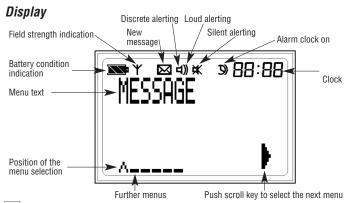
Field strength indication (this feature requires periodic sending of messages) If the receifer is out of range, the field strength indication in the display is visible.
