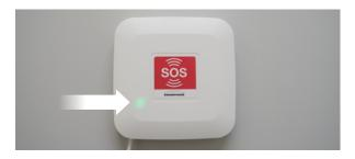
As soon as the beacon is powered by the power supply unit, a green light is visible. If there is no power supply from the power supply unit, the indicator goes out.
