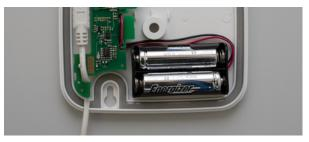
Remove the old batteries and place the new, full batteries in the battery compartment, where the correct battery polarity is indicated.
